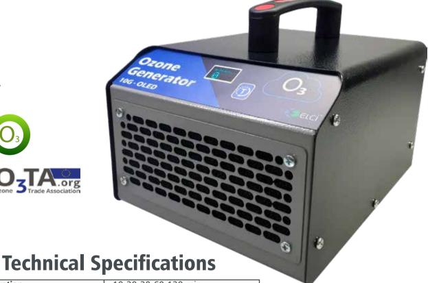
Set duration 10-20-30-60-120 min. Life-span of ozone sheets 5 000 hours 10 000 mg **Ozone Capacity** 220 V Voltage 128x64 0,96" oled Display **Operating Temperature** 8 - 49°C Weight 2,9 kg **Dimensions** 18,5 cm X 25,5 cm X 19 cm **Package Dimensions** 23cm X 24cm X 37cm
